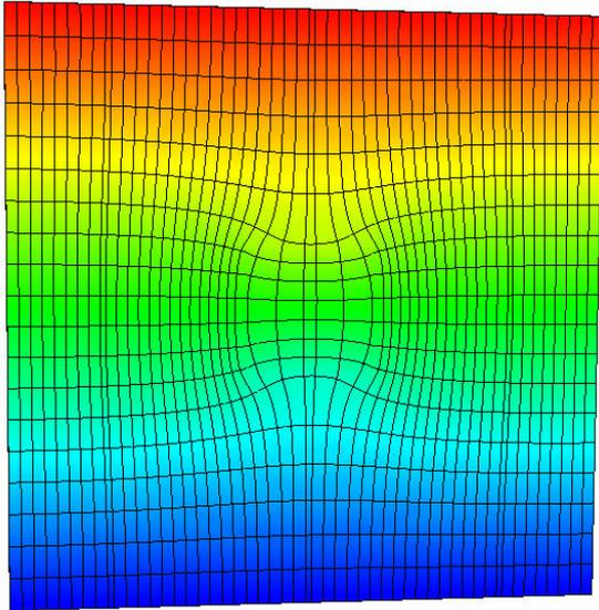
Figure 2. A single frame from an animation showing two dimensional conductive heat transfer. The central core has a thermal conductivity four times greater than its surroundings.
